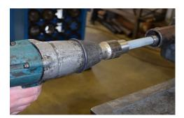
3 Disassemble the screw socket for the top expander (thread counter-clockwise), shear on the screw sleeve for the Thorbolt packer (long socket).
