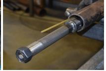
4 Expand the Thorbolt packer with the screw socket by turning the nut under the packer clockwise (right hand), use a nut runner.
