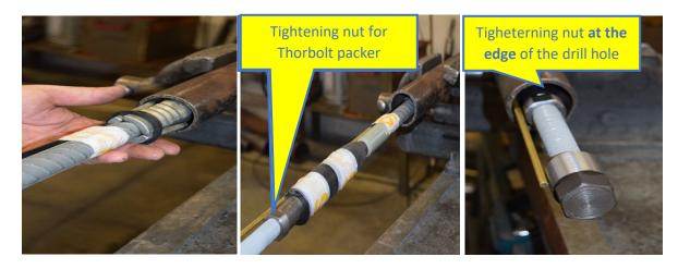
2 Tighten the top expander by turning the entire Thorbolt clockwise (right hand), using a nut runner.
