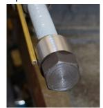
Adjust the top expander so it fits into drill hole and insert Thorbolt so <u>Thorbolt Packer tightening nut</u> ends up at edge of drill hole.
