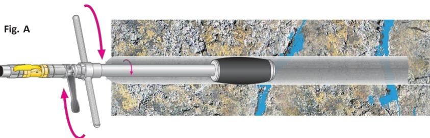
Insert the packer and expand the rubber sleeve in the hole either manually (as in the picture) or mechanically (with a wrench or nut-runner).
