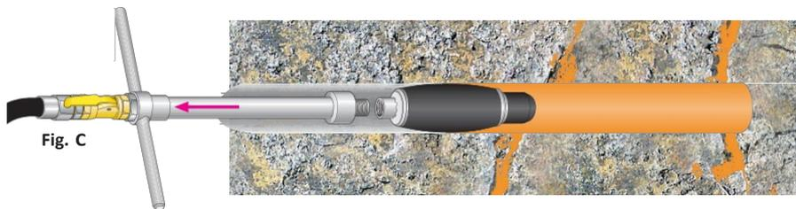
After grouting, remove the grout pipe for cleaning and reuse.
